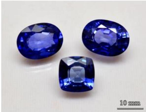
Figure 1. These examples of diffused synthetic sapphires range in size from 7.01 to 10.46 ct, showing strong blue colors. Photo by P. Ounorn
